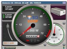
3. Click on Laser Start, verify laser is at 60mW (takes 10-20 seconds – the needle should move to the desired power on the gauge). You may need to click on Laser STOP first followed by Laser START for the laser to come on.
