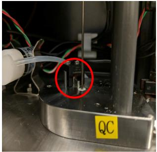
3. Use a small, thin object to push the small metal part down. **!!DO NOT TOUCH ANY OTHER** PARTS IN THIS AREA OR INSIDE THE MACHINE!!
