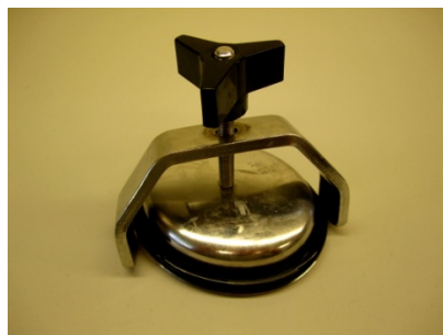
Correct- O-Ring Placement
