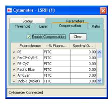
Adjust compensation in BD FACSDiva software either automatically using the compensation setup feature, or manually. When compensation is calculated using compensation setup (see Using Compensation Setup on page 137), you should not need to adjust the values after calculation.
