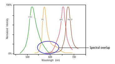
When the emission of one fluorochrome is detected by a detector designated for another fluorochrome, it is impossible to separate the two signals optically. The following example illustrates PE spillover into the APC detector.
