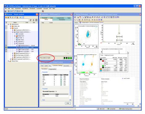
To verify that the workstation has successfully connected to the cytometer, check that the cytometer window displays the message *Cytometer Connected* or *The system is ready* at the bottom of the window. If the message is *Cytometer Disconnected*, see Electronics Troubleshooting on page 270 for assistance.
