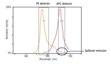
Compensation is the correction applied to the raw data to remove the effects of this spillover emission (ie, fluorescence). For example, when you are measuring
