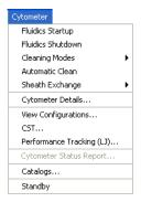
• Use the Cytometer window to view workstation connectivity status. When the software is connected to the cytometer, status messages are shown in the window. If an experiment is open and the current tube pointer is set, the window displays cytometer settings and laser controls for the current acquisition tube.
